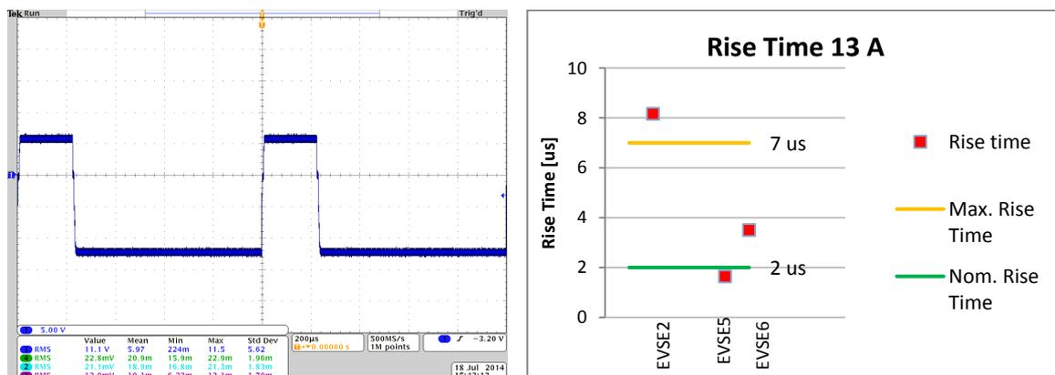
Figure 2 Measurement of an EVSE during round robin tests (13 Amp, state C),
