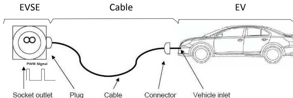
Figure 1 Physical components of the charging system
